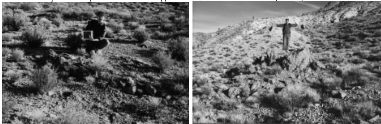
Figure 13: Field verification of spectral mixing results. Left photo shows an approximately 1 x 3 meter outcrop of dolomite found using sub-pixel detection. Right photo shows approximately 3 x 3 meter outcrop of dolomite.
