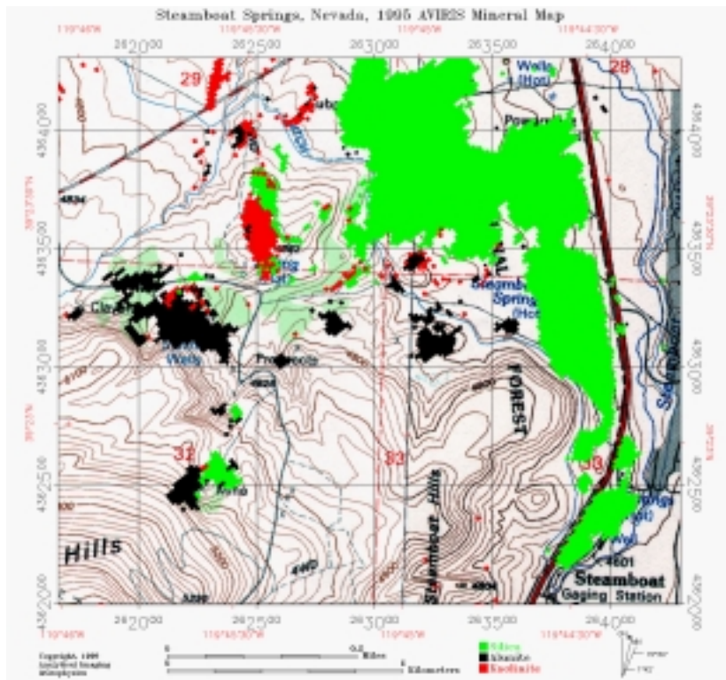
Figure 6: Steamboat, Nevada, 1995 AVIRIS mineral mapping results
