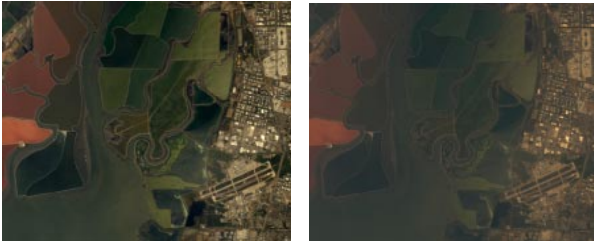
Figure 3. AVIRIS Moffett Field scene (left) and simulation with a 5 km visibility urban aerosol (right).
