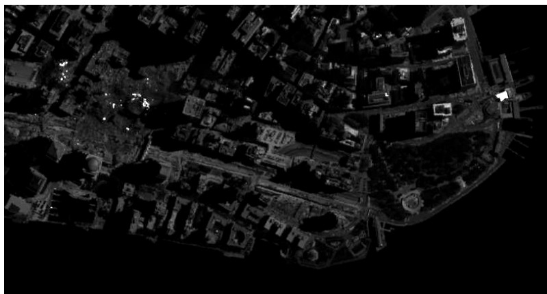
Figure 2. AVIRIS 2300-nm wavelength image of the World Trade Center disaster site. The bright signal to right side of the image is sun glint from a reflective roof surface.
