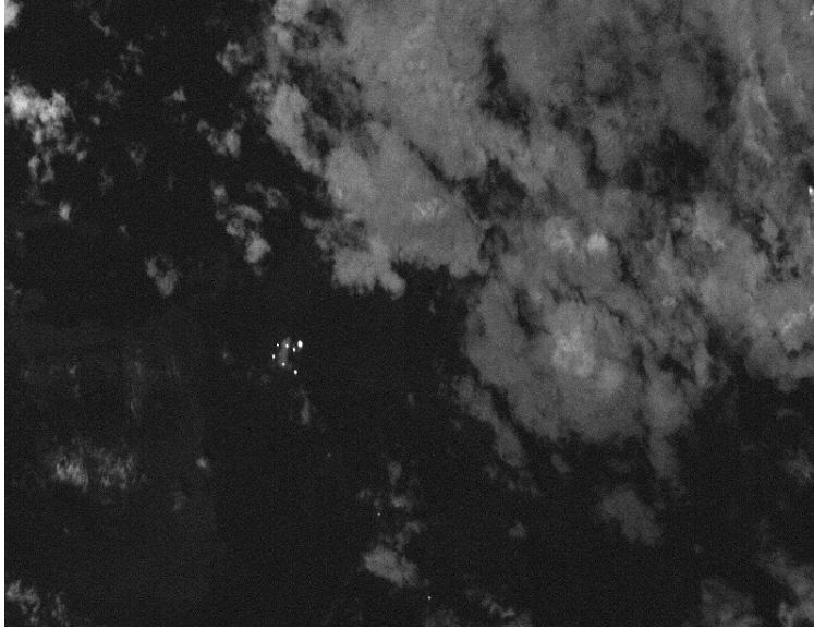
Figure 6. AVIRIS image at 2500.9 nm showing the emitted radiance of the hot lava.
