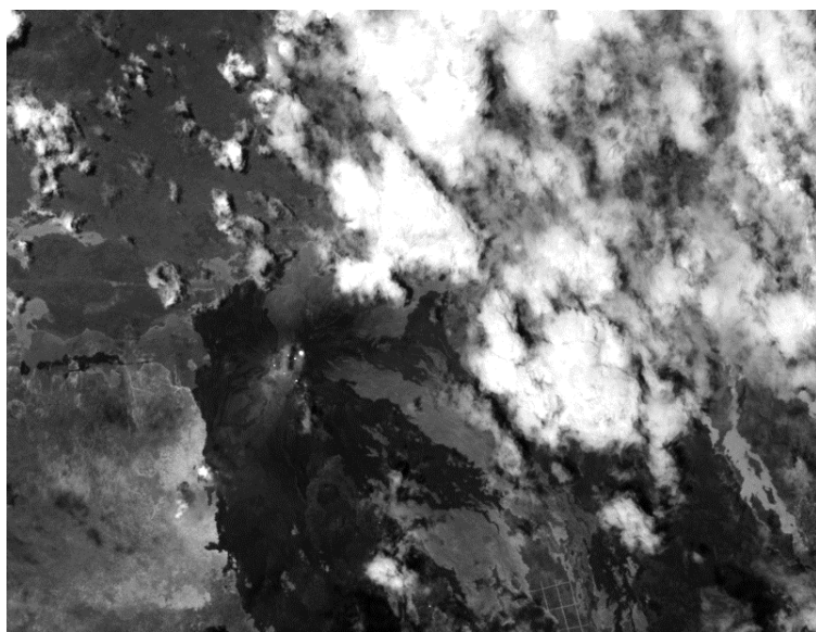
Figure 5. AVIRIS image at 1503.4 nm showing mixture of solar reflected radiance and hot target radiance from the active volcanic vent.
